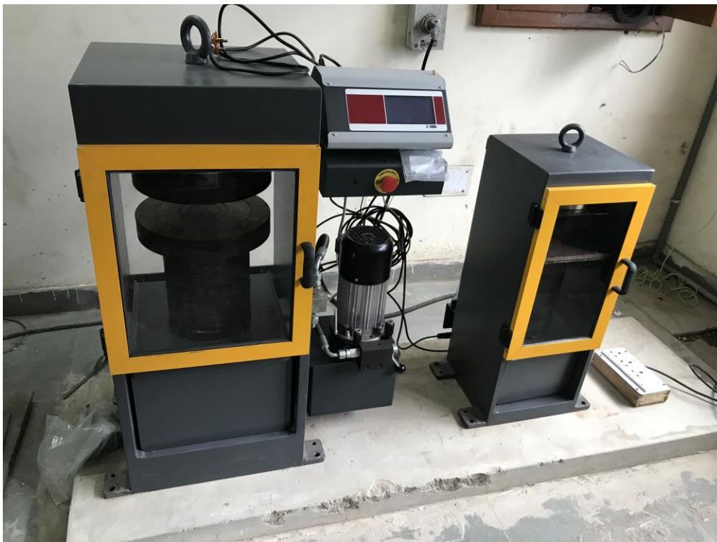
FULLY AUTOMATIC COMPRESSION TESTING MACHINE WITH TWO LOADING FRAMES 3000 KN AND 500 KN
