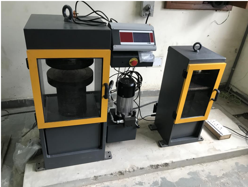
FULLY AUTOMATIC COMPRESSION TESTING MACHINE MAKE CONTROLS ITALY WITH TWO LOADING FRAMES 3000 KN AND 500 KN
