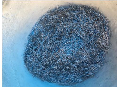
DOUBLE HOOKED STEEL FIBRE USED IN CONCRETE
